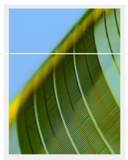
Flexing silicon's power: Arrays of tiny silicon solar cells like the one in this photograph are assembled using a transfer-printing technique. These arrays are as efficient as conventional solar cells, which are bulky and rigid. Each microcell in the array is about 1.5 millimeters long and 15 micrometers thick.
