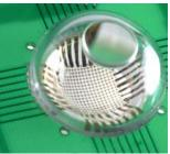
The eyes have it: This camera consists of a hemisphere-shaped array of photodetectors (white square with gold-colored dots) and a single lens atop a transparent globe. The curved shape of the photodetector array provides a wide field of view and high-quality images in a compact package. Credit: Beckman Institute, University of Illinois
