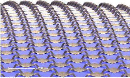
Stretchable mesh: The square silicon photodetectors, connected by thin ribbons of metal and polymer, are mounted on a hemisphere-shaped rubber surface. The entire device is able to conform to any curvilinear shape due to the flexibility of the ribbons that connect the silicon islands.
