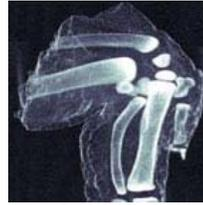
Researchers at the Paul Scherrer Institute (PSI) and the EPFL in Switzerland have developed a novel method for producing dark-field x-ray images at wavelengths used in typical medical and industrial imaging equipment. Dark-field images provide more detail than ordinary x-ray radiographs and could be used to diagnose the onset of osteoporosis, breast cancer or Alzheimer's disease, to identify explosives in hand luggage, or to pinpoint hairline cracks or corrosion in functional structures.
