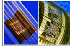
The so-called "nanonet" technology - circuits made of numerous carbon nanotubes randomly overlapping in a fishnet-like structure - has been plagued by a critical flaw: The network is contaminated with metallic nanotubes that cause short circuits.
