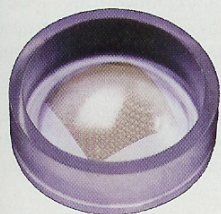
Formed into a shape reminiscent of a retina (inset), and mounted onto a rotatable stage, the flexible focal plane array acquires curvilinear images that can be flattened by software.
