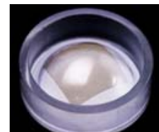
Silicon focal plane array (brown) and electronics on a hemispherical transfer element (translucent). Credit and Larger Version
