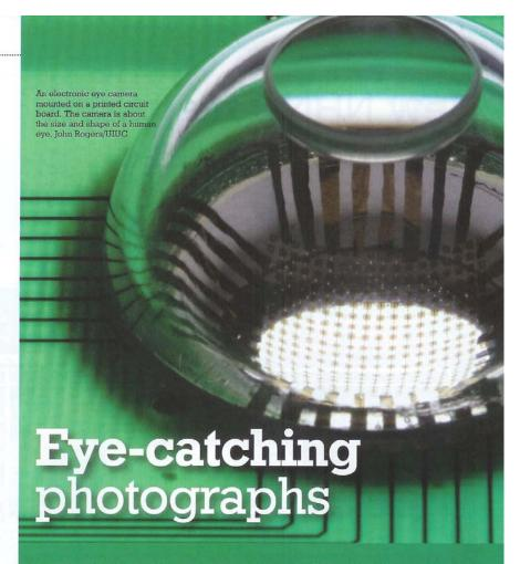
SCIENTISTS HAVE DEVELOPED AN EYE-SHAPED CAMERA USING A FLEXIBLE WEB OF MICRO-SENSORS. RATHER THAN USING A LIGHT SENSOR FOR THE CAMERA, THE TEAM DEVELOPED A SENSOR FROM A FLEXIBLE MESH OF WIRE-CONNECTED PIXELS. UNLIKE A NORMAL SENSOR MADE FROM A FLAT MICROCHIP, THE NOVEL MATERIAL IS ABLE TO CONFORM TO DIFFERENT SHAPES, SUCH AS CONVOLUTED, IRREGULAR SURFACES.
