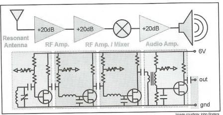
Block and circuit diagrams of a radio that uses carbon nanotubes for the resonant antenna, two radio-frequency amplifiers, radio-frequency mixer and an audio amplifier.
