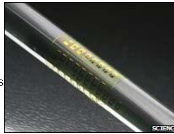
The silicon circuits can be wrapped around curved surfaces
