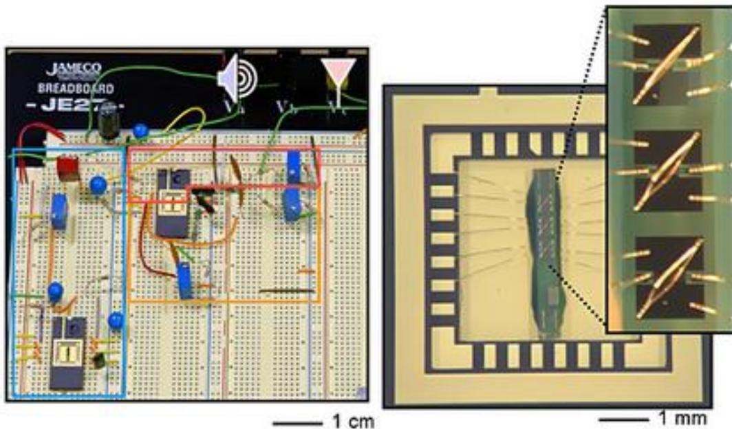
Image of the nanotube-transistor radio, which magnified views of carbon-nanotube transistors wire bonded into dual in-line packages.
