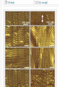
Silicon waves: A thin film of silicon has been affixed to a prestretched sheet of rubber. When the strain on the rubber is released, the silicon buckles to form a herringbone pattern. After the initial pattern has been created, the silicon and rubber are horizontally and vertically stretched and released.
