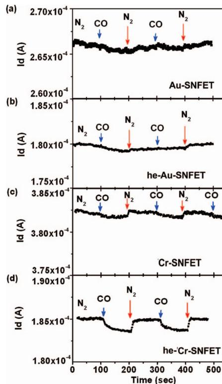
**Figure 2.** Electronic detection of CO gas using (a) Au-SNFET, (b) he-Au-SNFET, (c) Cr-SNFET, and (d) he-Cr-SNFET. The concentration of CO was 4.9 ppm and the total flow was kept at 500 sccm,  $V_g = 10$  V and drain voltage ( $V_d$ ) =  $-10$  V.
