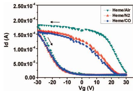
**Figure 3.** Transfer characteristics for a he-Cr-SNFET measured, respectively, in air, N<sub>2</sub>, and CO. The concentration of CO was 4.9 ppm and the total flow was kept at 500 sccm, V<sub>d</sub> = 5 V.
