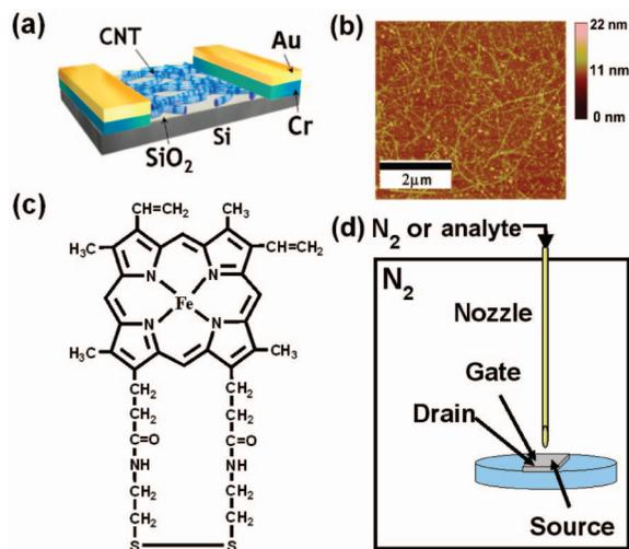
**Figure 1.** (a) Schematic illustration of the Cr-SWNT contacted SNFET. (b) AFM image of the SWNT networks. (c) Chemical structure of the thiolated heme. (d) Schematic illustration of the setup for gas sensing.
