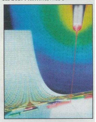
**E-jet printing** Electric-field induced jets of functional organic electronic inks from nanoscale nozzles forms the basis of a technique, which researchers refer to as e-jet printing, to pattern electronics on flexible substrates.
