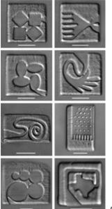
**VARIETY** Mask-based multiphoton lithography generates numerous shapes (scale bars =  $15 \ \mu m$ ).
