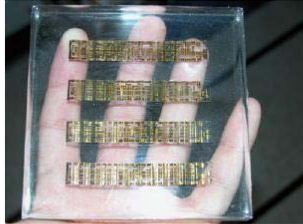
Hands-on mock-up of a stretchable silicon transistor-- part of the Nano-CEMMS traveling exhibit
