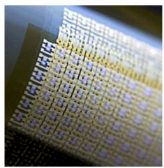
A new method of printing layers of high-performance transistors on a sheet of plastic could lead to flexible electronics.
