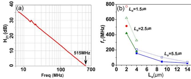
Fig. 4. (a) Experimental plots of  $H_{21}$  obtained from TFT of  $L_c = 2 \mu\text{m}$  and  $L_o = 1.5 \mu\text{m}$  with  $V_g = 2 \text{ V}$  and  $V_d = 2 \text{ V}$ . (b) Dependence of  $f_T$  on the gate length of TFTs: Measured (filled) and calculated values (open).
