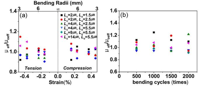
Fig. 3. (a) Normalized effective mobility ( $\mu_{\text{eff}}/\mu_{0\text{eff}}$ ) as a function of bending-induced strain and bending radius. (b) Normalized effective mobility after bending (to  $3\text{-mm}$  radius;  $0.44\%$  strain) and unbending the devices several thousand times.
