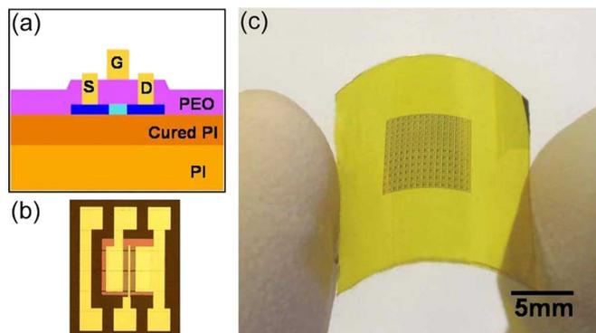
Fig. 1. (a) Schematic cross-sectional view of a single-crystal silicon TFT on PI (PI;  $25\text{-}\mu\text{m}$  thick) with a  $\text{SiO}_2$  layer deposited by low-temperature PECVD as a gate dielectric (PEO;  $100\text{-nm}$  thick). (b) Optical-micrograph top view of a typical device. (c) Optical images of an array of devices on a plastic substrate.
