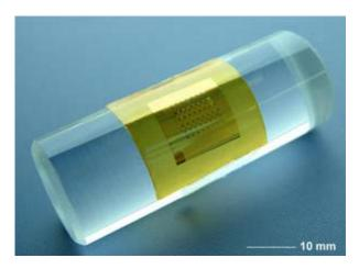
A key feature of the strategy is that it occurs at room temperature, thereby enabling the electronics to be placed on unconventional substrates such as thin sheets of plastic.
