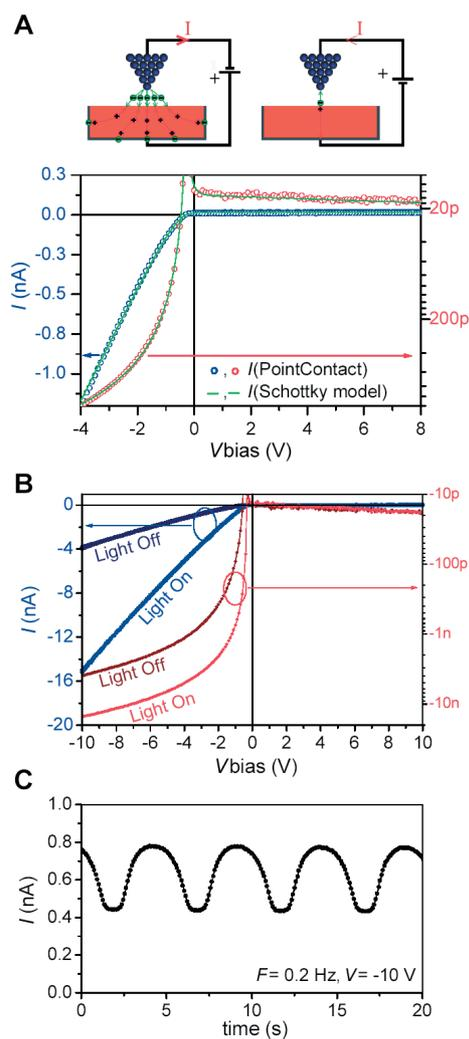
**Figure 4.** Rubrene bulk crystal point-contact diode. A) *I*–*V* characteristic of a rubrene point-contact diode (dots) fitted with the Schottky model (line). The top scheme illustrates the carrier injection mechanism at the tip and bottom electrodes of the point-contact diode. B) *I*–*V* characteristics of the device under white-light excitation. C) Time dependence of the forward-current amplitude upon exposure to a white light-emitting diode electronically modulated with a 0.2 Hz sinus wave.
