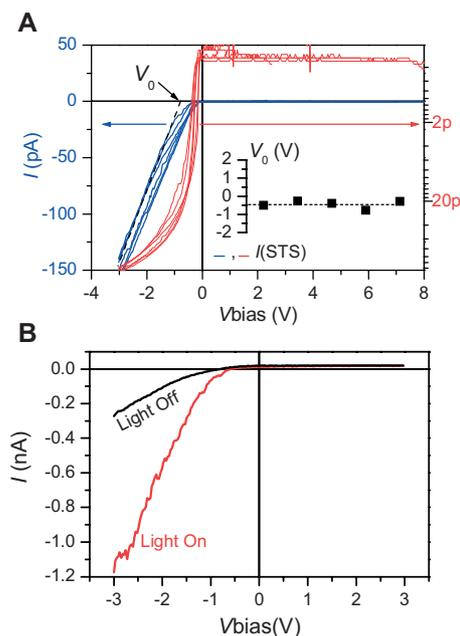
**Figure 3.** STS on the rubrene bulk single-crystal surface. A) *I*–*V* tunneling spectra of the tunnel diode presented on a linear (left) and logarithmic (right) axis showing the perfectly rectifying behavior of the p-type rubrene semiconductor. The inset plot shows the extracted turn-on voltages from the tunneling spectra. B) *I*–*V* tunneling spectra recorded in the dark and under white-light excitation at a different location on the rubrene crystal.
