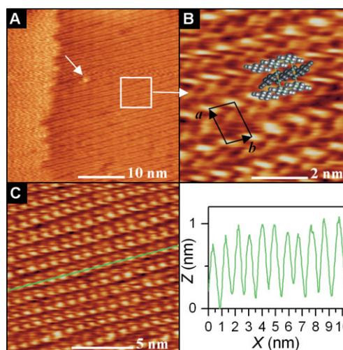
**Figure 2.** STM images of the rubrene surface. A) Typical large-scale STM image of the rubrene crystal surface in the constant-current mode ( $U_t = -1.065\text{ V}$ ,  $I_t = 29\text{ pA}$ ). B) A smaller-scale image ( $U_t = -1.138\text{ V}$ ,  $I_t = 29\text{ pA}$ ) reveals the herringbone organization of the rubrene molecules in the  $a$ - $b$  plane. C) Larger-scale image and cross-sectional profile along a single row of molecules in the  $b$ -axis direction of the crystal.
