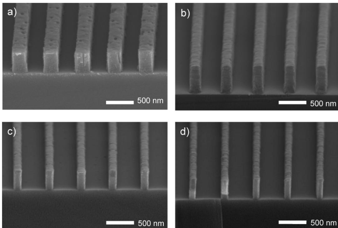
**Figure 3.** Cross-sectional SEM images of the resulting PDMS/SiO<sub>2</sub>/PL resist structures on Si(100) substrates after RIE of SiO<sub>2</sub> for (a) 35 s, (b) 40 s, (c) 45 s, and (d) 50 s and anisotropic etching of PL for 5 min.
