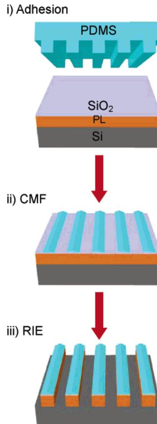
**Figure 1.** Schematic illustration of the procedure for preparing high-aspect-ratio resist structures on a silicon substrate using a combination of CMF and RIE.
