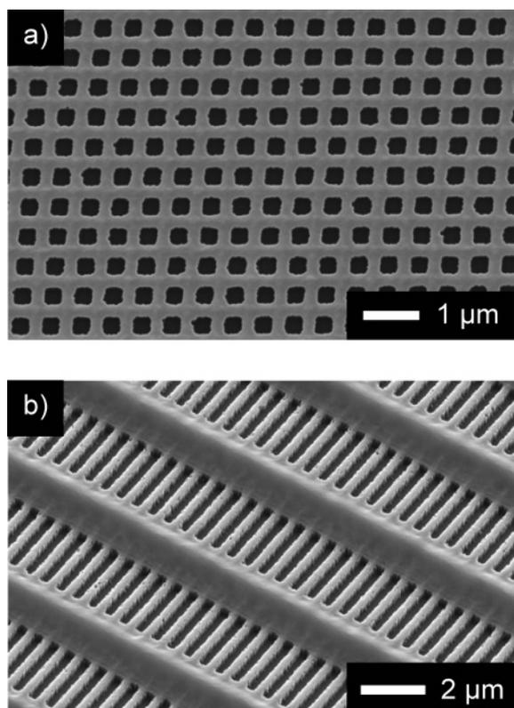
**Figure 4.** Top-view (a) and tilted-view (b) SEM images of the multiply transferred PDMS lines after RIE of SiO<sub>2</sub> and PL layers. 300 nm (a) and 2 μm (b) wide line patterns have been used for the second set of PDMS lines.
