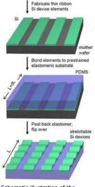
Schematic illustration of the process for building stretchable single crystal silicon devices on rubber substrates.
