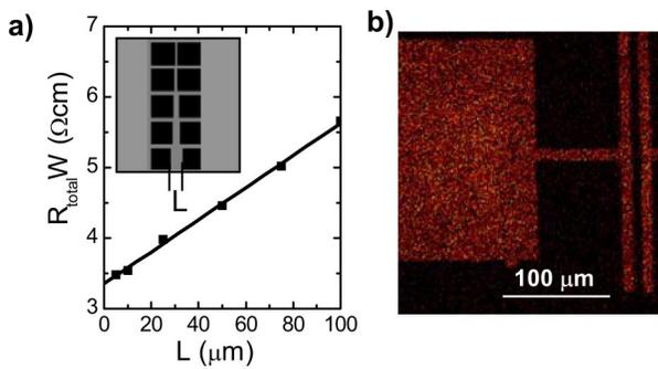
FIG. 2. (Color online) (a) Width normalized resistance ( $R_{\text{total}}W$ ) measured between two contacts as a function of  $L$  on uniform, highly doped  $\mu\text{s-Si}$  thin film. The intercept of a linear fit to these data gives a contact resistance. Inset shows the test structures for evaluating the contact resistance; (b) phosphorus concentration in a silicon film with patterned doping, as evaluated by TOF-SIMS.
