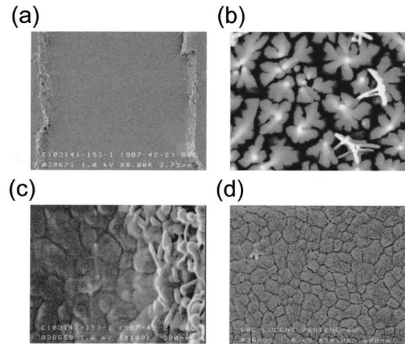
FIG. 3. (a) Scanning electron micrograph (SEM) of a  $10$   $\mu\text{m}$  channel with printed DNNSA-PANI/SWNT source and drains at the edge; (b) AFM of a region in the middle of the channel of a pentacene transistor that uses printed DNNSA-PANI/SWNT electrodes like those shown in (a); (c) SEM of the pentacene grains at the source/channel interface; (d) SEM of a Au electrode on pentacene.
