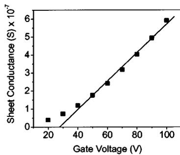
FIG. 8. Sheet conductance of the channel region as a function of gate voltage as derived from data in Fig. 7. The slope and  $x$ -intercept of the fitted line give an intrinsic mobility of  $0.68 \text{ cm}^2 \text{ V}^{-1} \text{ s}^{-1}$  and an intrinsic threshold voltage of  $27.7 \text{ V}$ , respectively.
